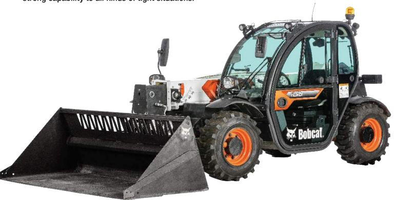
Its 72.1-inch width, four steering modes, and two-stage, low-profile boom change the game in places other machines won't fit. Tackle tricky material handling between buildings and obstacles or take advantage of a wide array of Bobcat attachments for maximum versatility.
