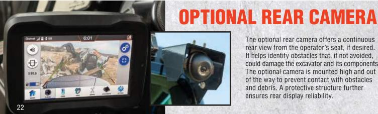
The optional rear camera offers a continuous rear view from the operator's seat, if desired.
