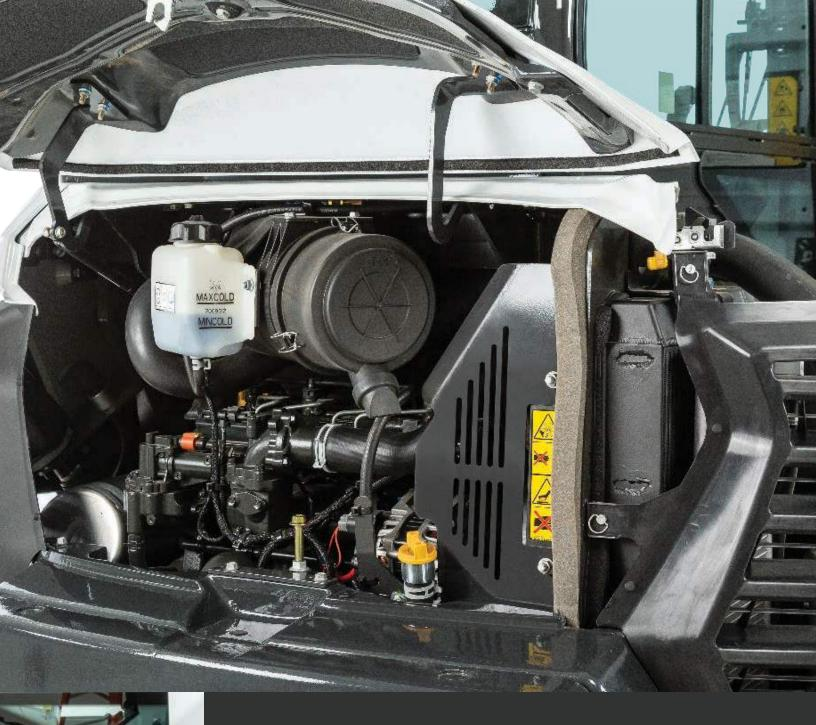
Bobcat makes it easy to find and reach your engine checkpoints in a Bobcat excavator so daily maintenance actually gets done every day. Comparing our service access to other excavators is like comparing a 60-inch LCD to a 15-inch black-and-white TV. The swing-open tailgate and side access hood put the engine and pump package, valve bank, cooling system, and plumbing in easy reach.
