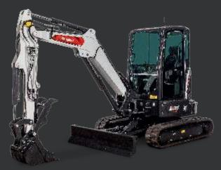
33.2 hp (24.7 kW) Standard, Long or Extendable Arm 121.2 in. (3077 mm) – 153.2 in. (3892 mm) Dig Depth
